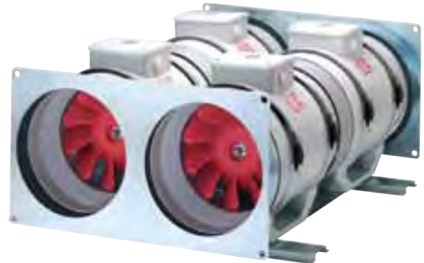
IN SERIES + PARALLEL FOR RECTANGULAR DUCTS (DOUBLES THE PRESSURE AND THE AIR FLOW)
